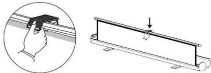
5. Close the casing and rotate the left & right support plate (Stand holder) inwards and align them with the casing.
