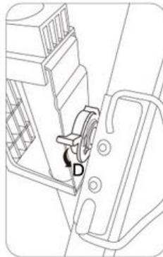
5. With the dial knob on the handle hatch, it is possible to remove the entire housing case of the screen. This is done by turning the dial knob downwards as shown on the picture.
