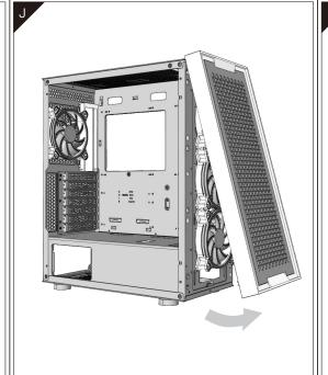
Remove the front panel of the case and open it by hand in the lower direction
