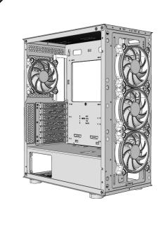
Front: 3 x 120mm fan(included) Rear:1x 120mm fan(included) Top:2 x 120 /140mm fan(optional)
