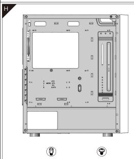
According to the motherboard model, Main board screws are used for fixing copper column should be replaced manually Support E-ATX/ATX/M-ATX/Mini-ITX
