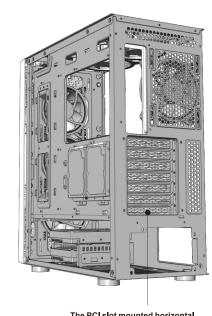
The PCI slot mounted horizontal
