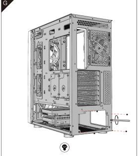
The power supply can be fixed by aligning the screw in the figure to the hole position
