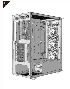
WaterCooling System:Front:1 x 240/360mm Top:1 x 240mm Rear:1 x 120mm
