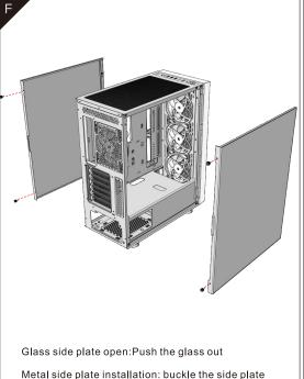
Metal side plate installation: buckle the side plate and fix it with two screws
